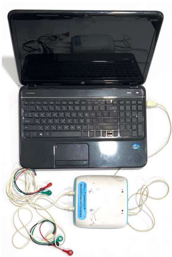
Figure (1) sEMG ( Neutostyle, Pte. Ltd) device.
